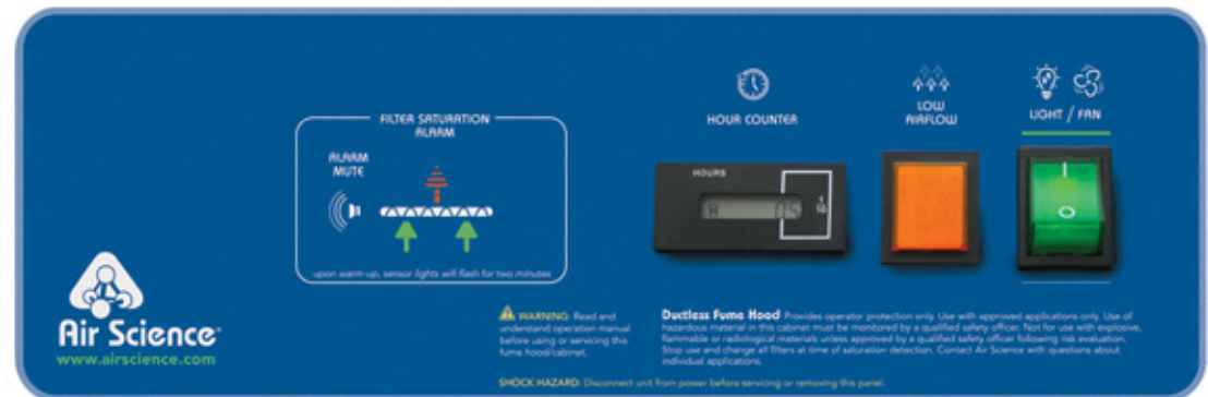
Optional Advanced control panel with hour meter to aid in determining available filter life and Filter Saturation Alarm (FSA) . The FSA adds an electronic gas sensor and emits audio and visual alerts when the main filter needs to be changed.
